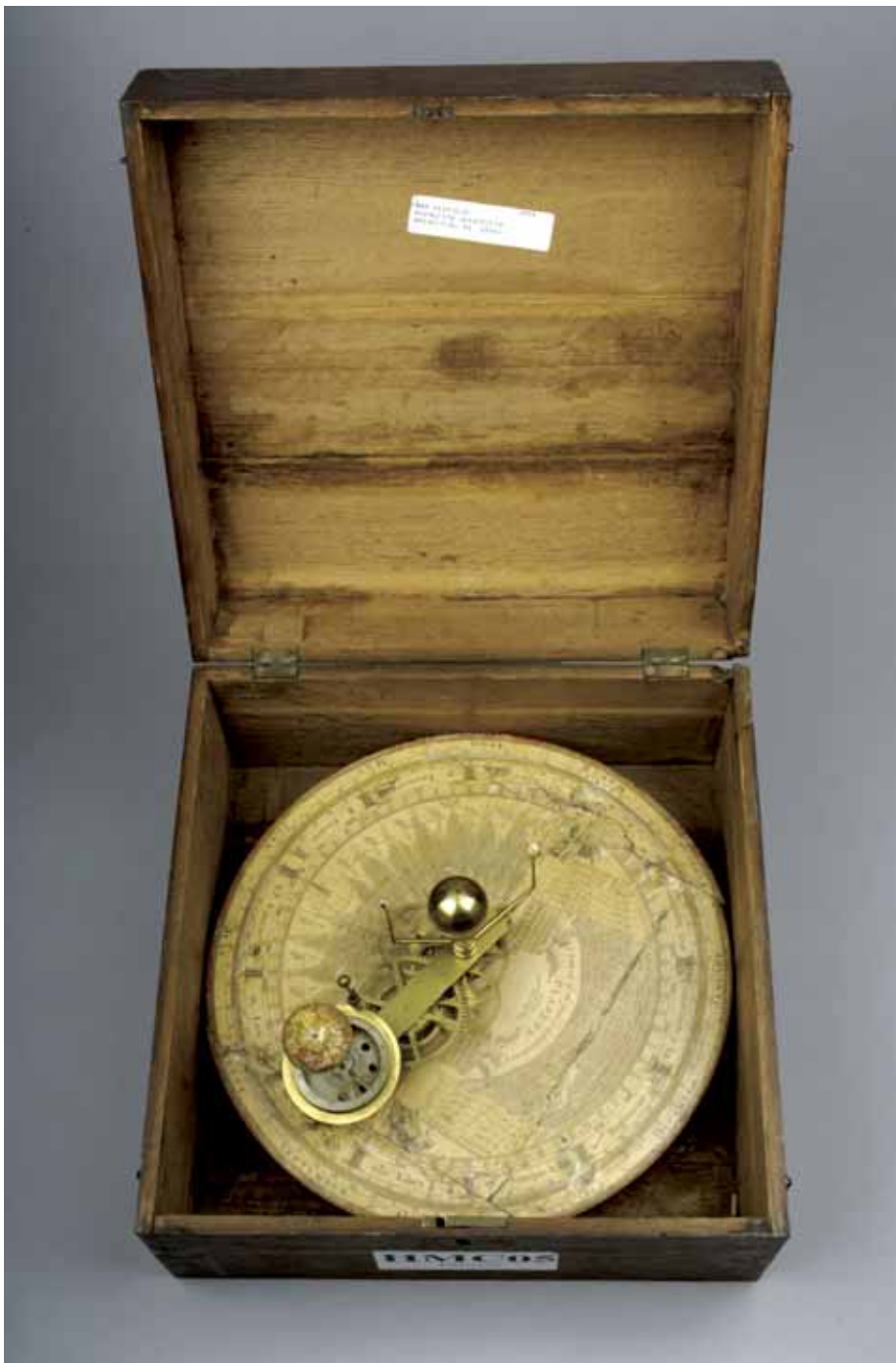
Hand-cranked orrery, showing the movements of Mercury, Venus, and the Earth around the Sun, and the Moon around the Earth. Printed, colored, and varnished dial; brass wheels and gears, Sun and Moon; ivory planets. Built by famed London instrument makers, William and Samuel Jones, 1794. The orrery demonstrates astronomical phenomena related to the diurnal rotation of the earth, the annual revolution of the earth around the sun, and monthly revolution of the moon around the earth, such as the reasons for day and night, seasons, and eclipses. The dial has calendar, zodiac names, symbols, and figures, and related calibrations in the outer concentric circles; tables of data relating to the planets (Mercury through Saturn) occupy the center area. Image courtesy Historic Maps Collection, Department of Rare Books and Special Collections, Princeton University Library.
